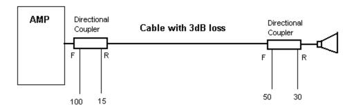
While the cable loss can be added into the measurement, it is more accurate to make the measurement at the input of the device in question. The reason is that every connection or device along the way can have its own VSWR.
